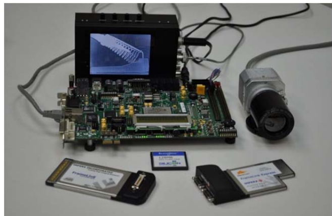
Figure 31. RIDL-Link hardware and software platform for multi-interface video acquisition
