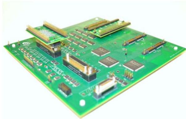
Figure 53. This image shows a cryogenic multi-layer circuit board designed in the CfD and populated in CEMA. All of the components on this board will be exposed to temperatures as low as 40 K, nanoTorr pressure levels, and high energy particle radiation.
