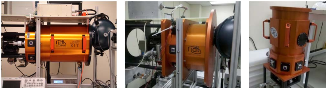
Figure 49. Detectors are evaluated in three custom dewar test systems.
