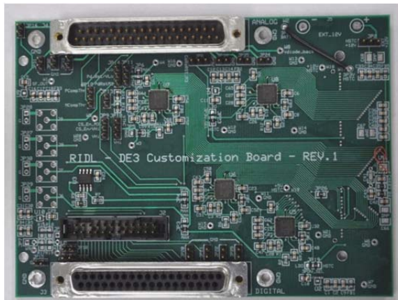
Figure 30. Low-noise data acquisition board for use with the NASA Low-Noise Imaging Detectors.
