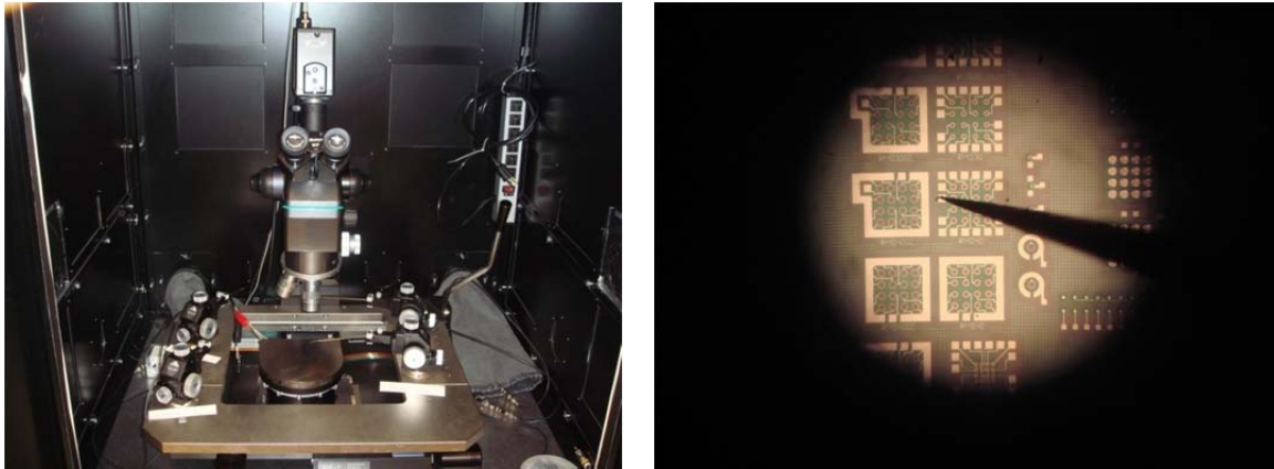
Figure 8. (left) The Rochester Imaging Detector Laboratory cleanroom probe-testing station. (right) a LIDAR-style GM-APD wafer with a probe applied to a pad of a device.
